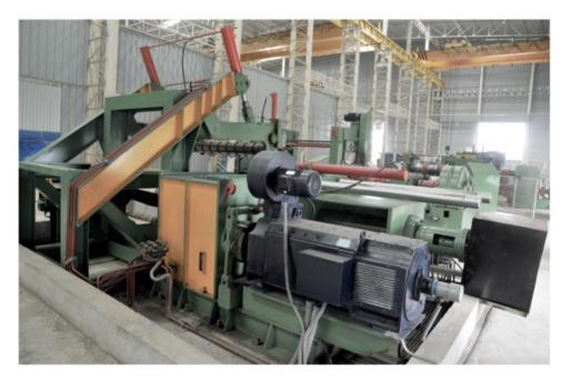
The newly-installed HR slitter will process coils up to 12-mm thick and 1650-mm wide into strips of desired widths down to 50-mm, which clearly is a benchmark in the country.
